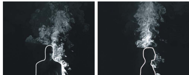
Fig. 8 Experimental PIV images of the particle-laden flowfield
