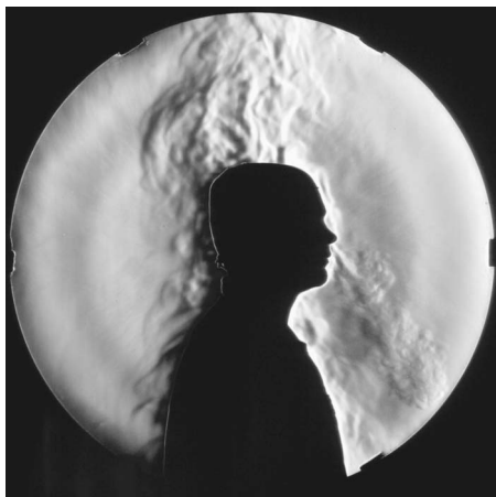
Fig. 2 Schlieren image of the human thermal plume, side view. Notice also the warm turbulent exhaled air from the nose of the subject.
